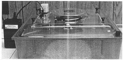
Fig. 23 "Roll-X" incubator.
