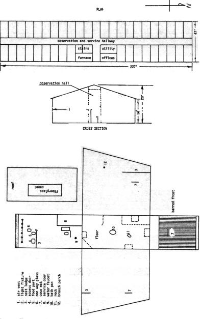
Fig. 42 Floor plan, elevations, and exploded view, Ithaca facility.
