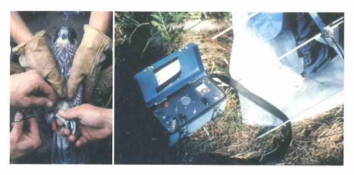
Figure 13. Transmitter placement and telemetry receiver.
